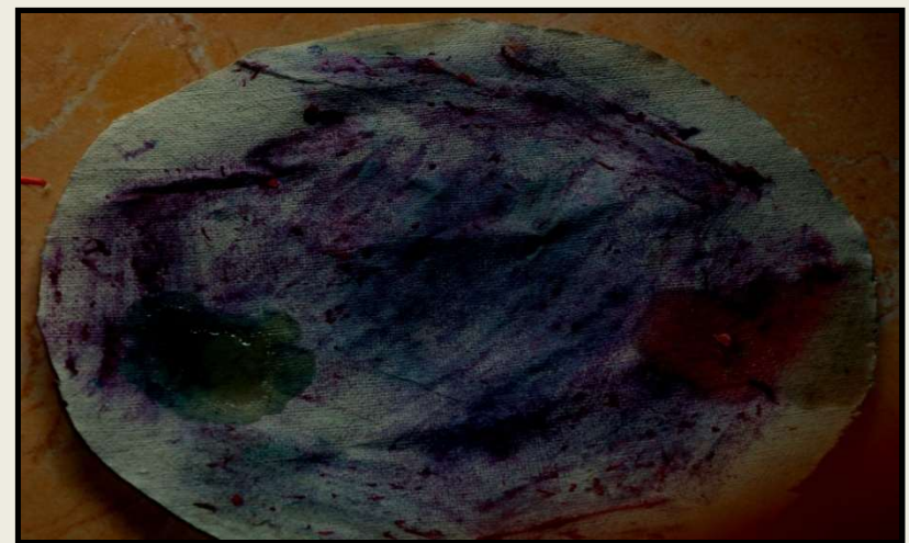
4. China rose indicator gives green colour with base and red with acids.
