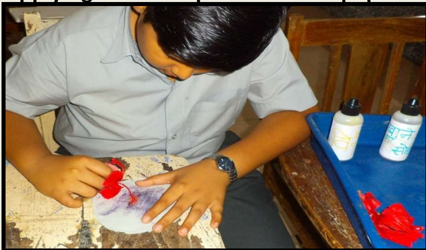
3. Preparing china rose indicator by rubbing china rose petals on filter paper
